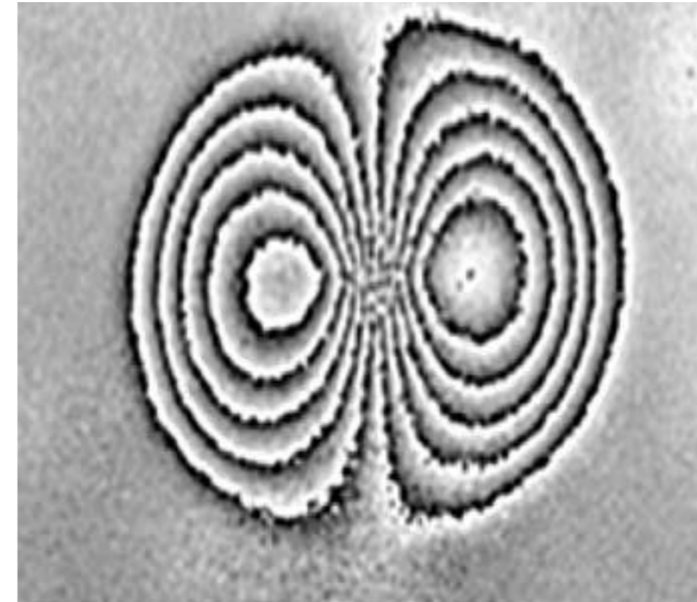
Shallow delamination in composite
