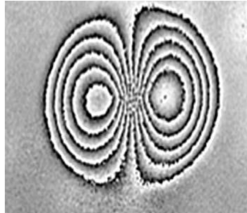
Shallow delamination in composite
